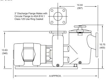
The pump-motor bracket shall incorporate the seal housing which shall have stationary diversion vanes to ensure a constant flow of fresh water past the seal. The 1.25 in. (32mm) dia. mechanical seal shall have stationary and rotating faces of ceramic and carbon respectively.
